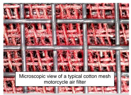
This is a photo of a cotton air filter. Yes, you can see the holes between the threads, and yes, the holes are pretty big, holes as big as 400x700 microns, the overlapping of many strata, in this case a street application of three layers, will try to make sure not too many holes are simply passing-through channels. No need to say more, right?
