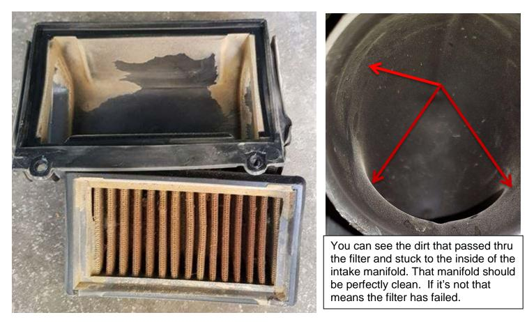
Fine and middle sized dust particle went through the filter, went inside the AIRBOX, and down the intake manifold. **THIS IS NOT ACCEPTABLE**. Yes the filter passed plenty of air (really far too much) and at the same time it passed plenty of dust too. Would you want this in YOUR engine? You tell me.
