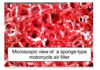
You see, a filter that uses an "oil trapping" technology allows "huge" particles to pass by the filter and go into your engine.
