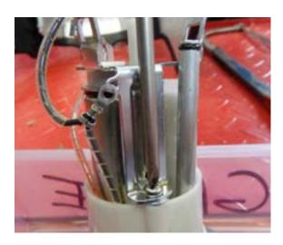
Remove the two screws which hold the fuel pump into the base of the fuel pump housing. Lift off the lower white plastic housing.
