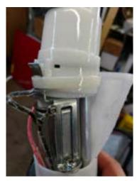
Failing to do so, if the assembly is not correctly repositioned, it will eventually pop open again due to fuel pressure. Install the provided large cable tie to push down the two metal lips and hold the whole assembly into position.
