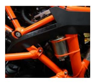
We can provide without extra costs a larger unit to be mounted on the frame, easier to access and to change for servicing, as always position it vertical with the "out" on top.
