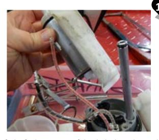
Lift the fuel pump out of the dark plastic base. The OEM filter is press fitted onto the base of the pump; remove and discard the OEM filter.
