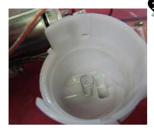
The Fuel System NEEDS A MAIN FILTER, either you will wash and re-use the paper original one, or you MUST INSTALL an In-Line ot ouf Tank Fuel filter. If you install the latter, the paper filter will be disposed of system. Remove and discard the OEM filter.
