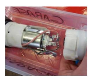
Once the fuel pump is completely removed from the tank, remove the plastic head of the fuel pump. There are two plastic tabs which need to be depressed before the plastic head can be gently removed.
