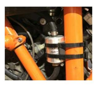
Once all parts are back in place, DO NOT switch the engine at once. Prime the system doing 5 times the std check, rotate the key, do the ingnition check and switch off, with each action you may notice a different sound from the pump, sign that it is bleeding out the air, on the 6th turn of the key, start the engin. You're GOOD TO GO.
