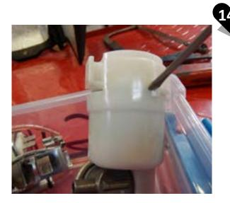
The OEM paper filter is located inside the plastic head. Use a small flat head screw driver to gently depress the plastic tabs shown in order to remove the lower half of the plastic unit and expose the paper filter.
