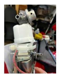
While closing back the upper part, install, always with a drop of engine fresh oil, the provided new o-ring. Close it properly paying attention to check many times the correct position both of the two halves and of the assembly on top of the fuel pump itself.
